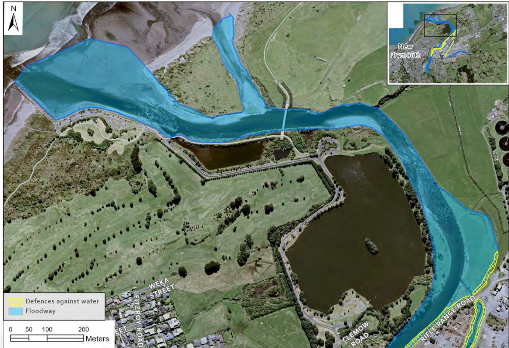
Map 3a Defences against water and floodways along the Waiwhakaiho River and Upper Mangone Stream, New Plymouth.
