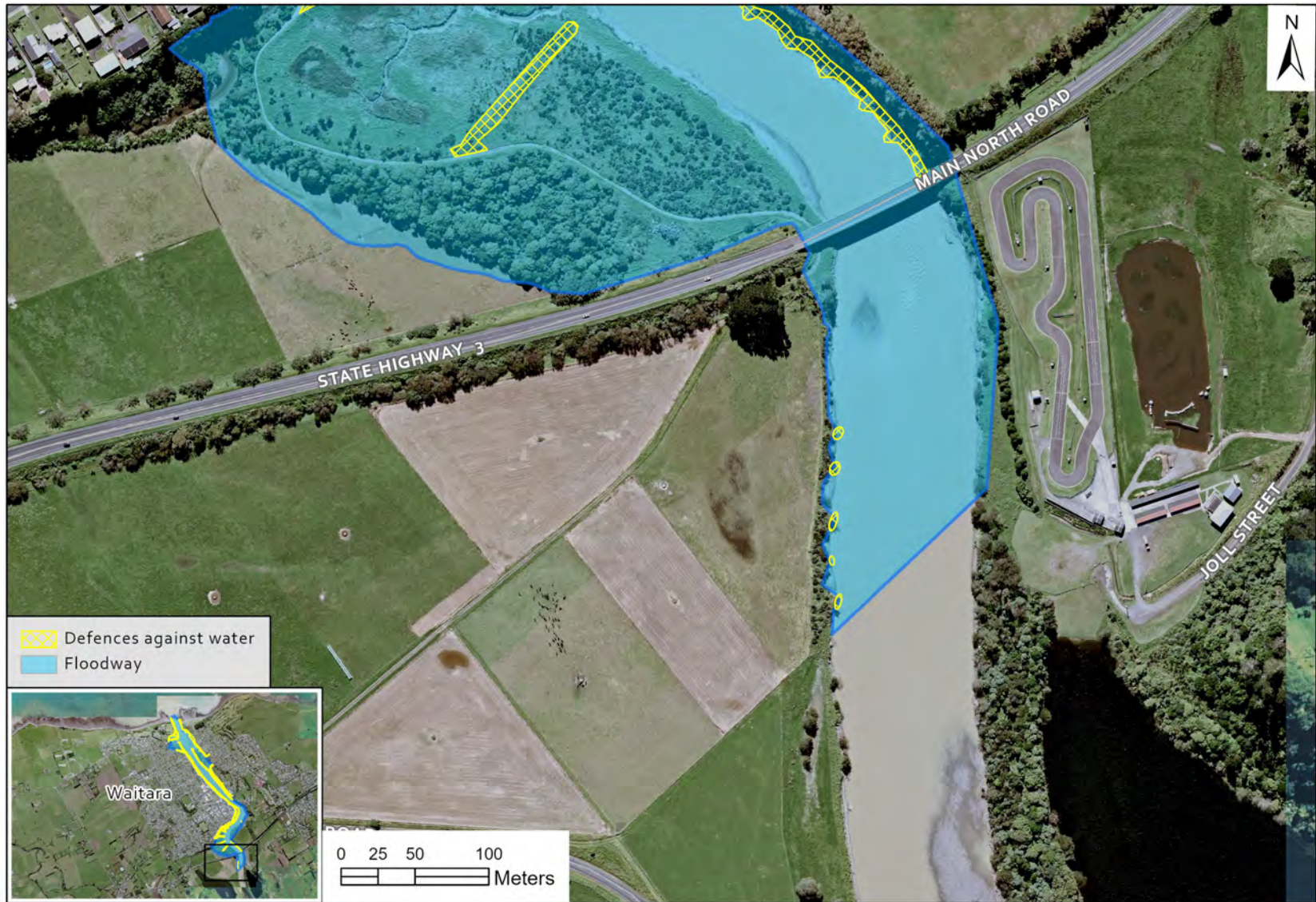
Map 2e Defences against water and floodways along the Waitara River, New Plymouth.
