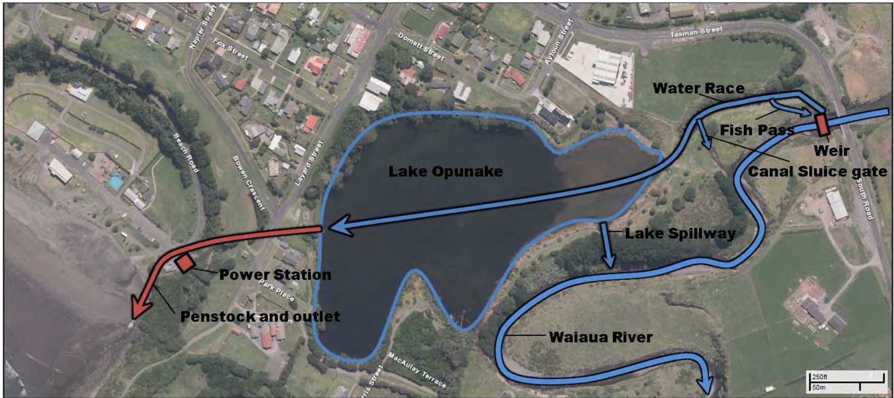
Photo 2 Opunake Power Limited scheme on the Waiaua River
