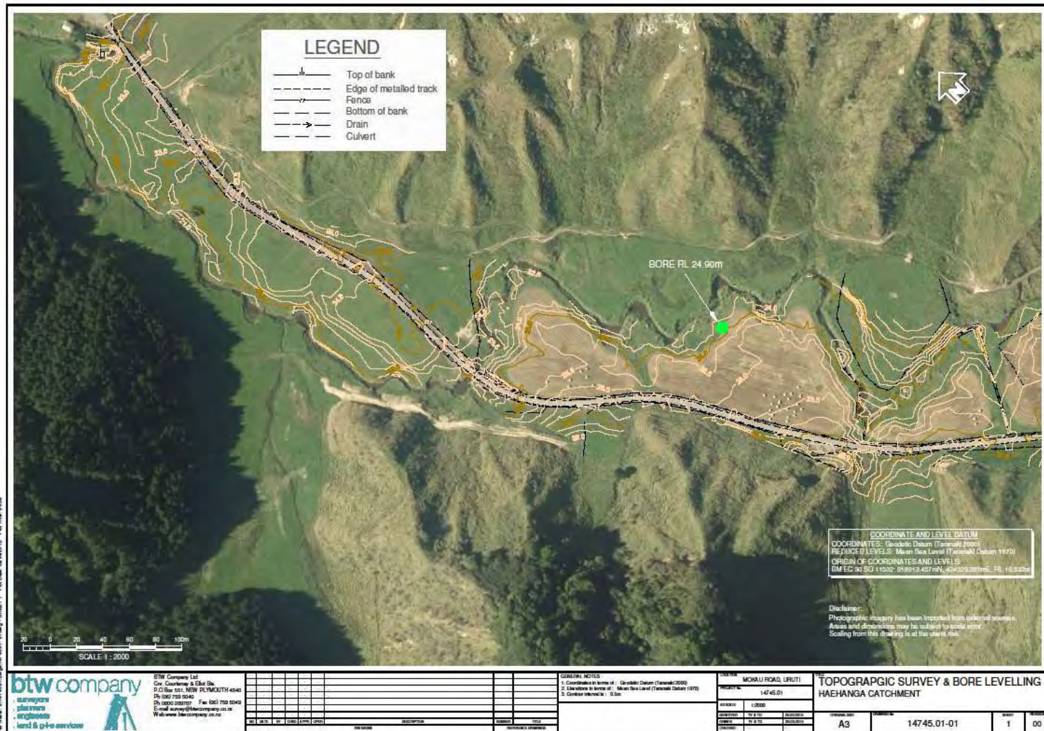
Figure 2.1:Uruti Composting Topography Survey-lower part of site. Green dot denotes GND 2190 and reduced level
