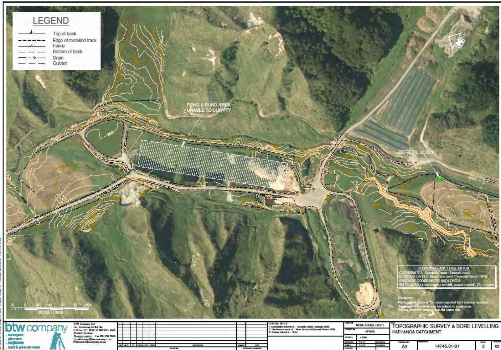
Figure 2.2:Uruti Composting Topography Survey-middle part of site. Green dot denotes GND 2189 and reduced level
