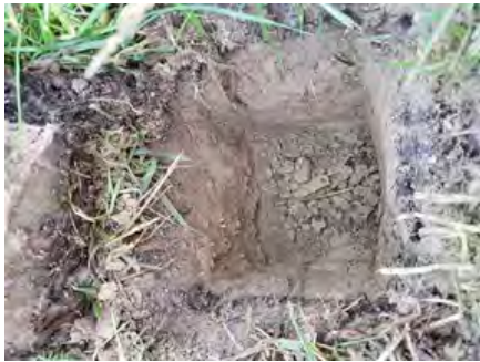
Figure 4: Photos showing test pit.
