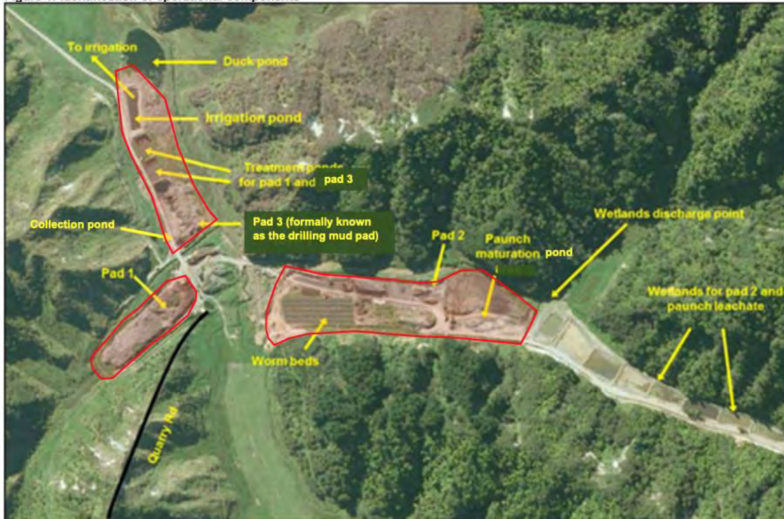
Figure 1: Identification of operational components
