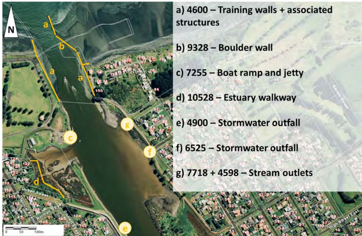
Figure 2 Indicative location of monitored coastal structures at Waitara
