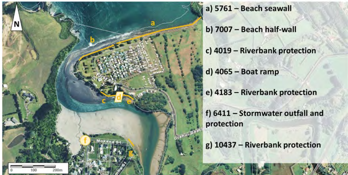
Figure 1 Indicative location of monitored coastal structures in Urenui
