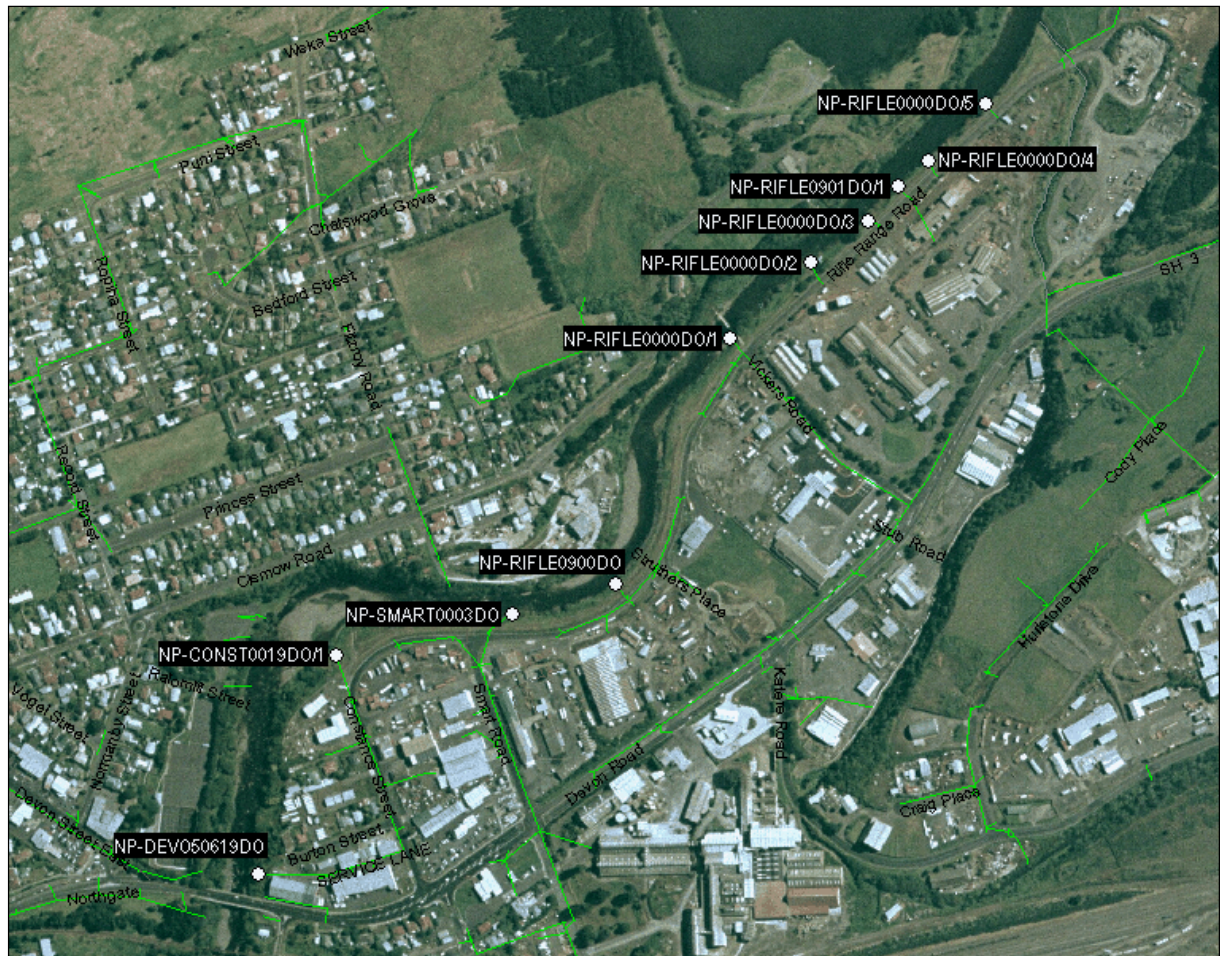
Figure 11 NPDC stormwater drainage and consented discharge points to the Waiwhakaiho River
