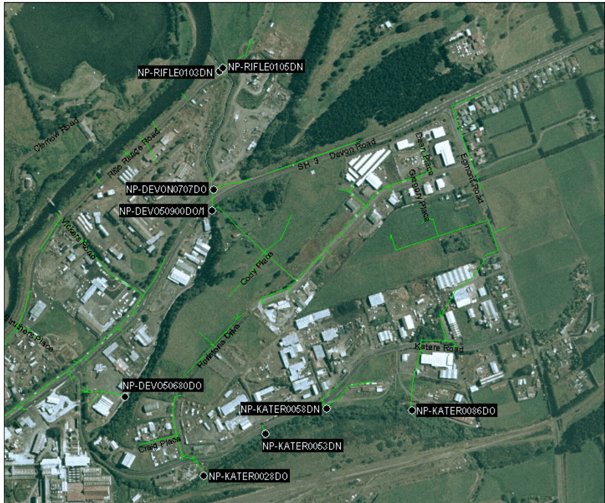
Figure 12 NPDC stormwater drainage and consented discharge points to the Mangaone Stream
