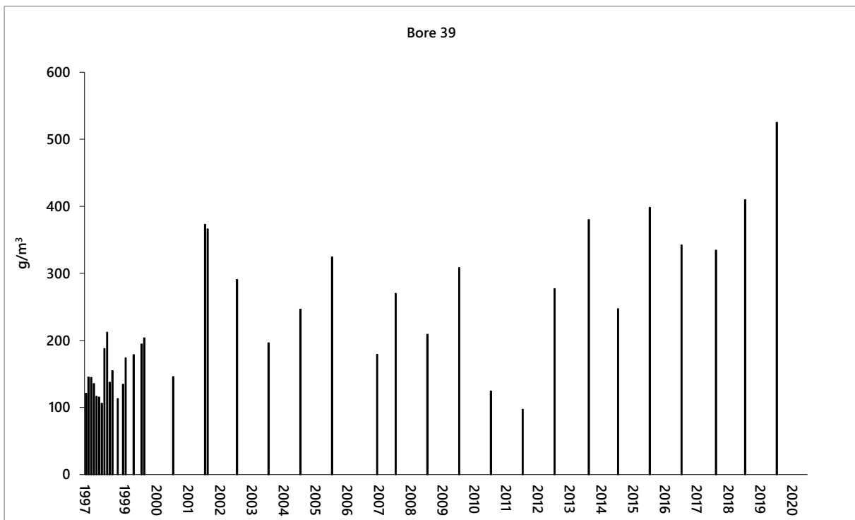
Figure 15 Total nitrogen concentration in groundwater near the urea processing areas from Bore 39
