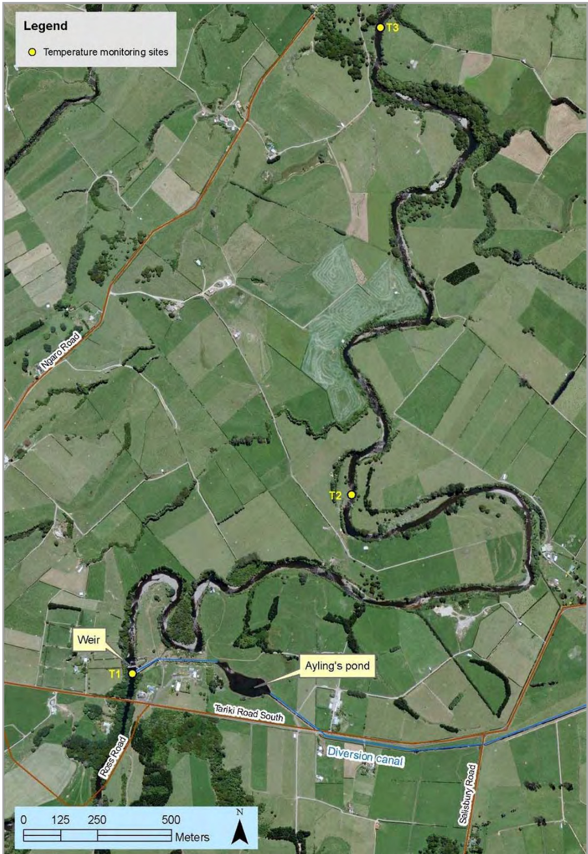
Figure 2 Continuous water temperature monitoring sites in the Manganui River in relation to the Motukawa HEP scheme
