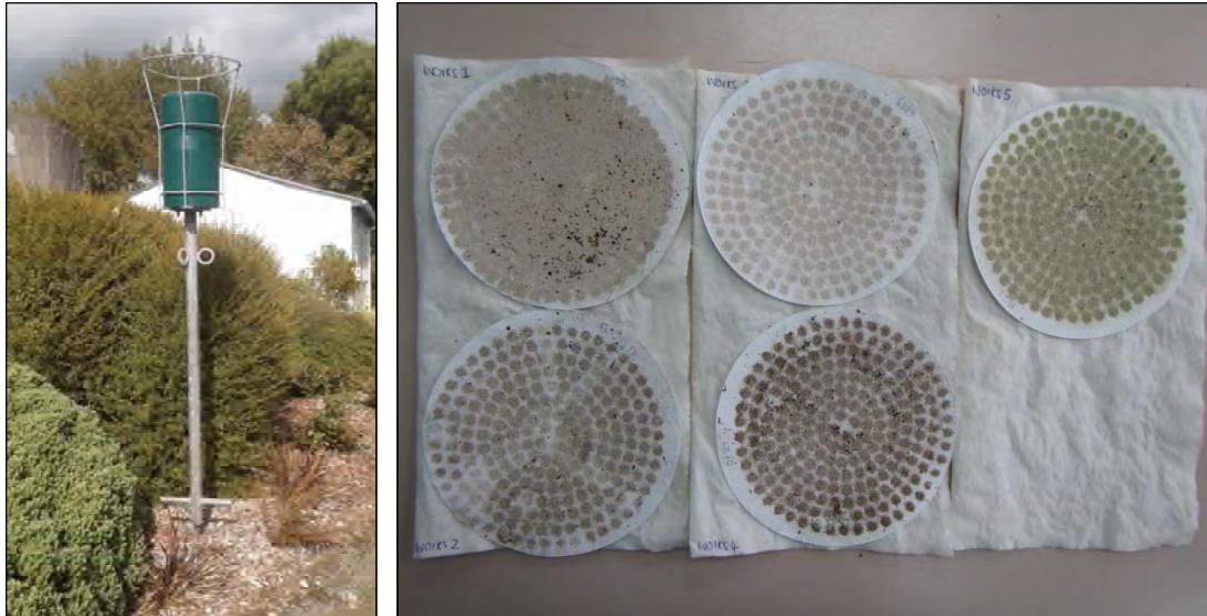
Photo 1 Examples of a deposition gauge set up and recovered filter pads
