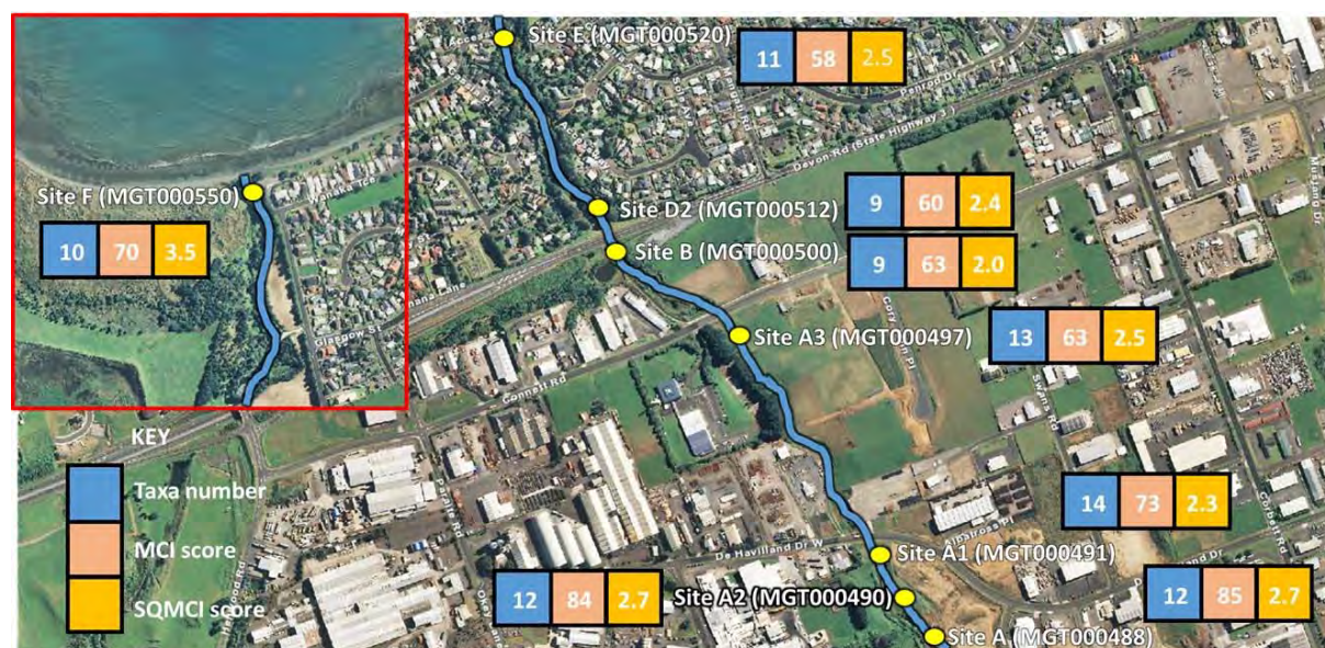
Figure 4 Biomonitoring sites in the Mangati Stream in relation to the Bell Block industrial area with taxa number, MCI scores and SQMCI scores for each site in October 2019
