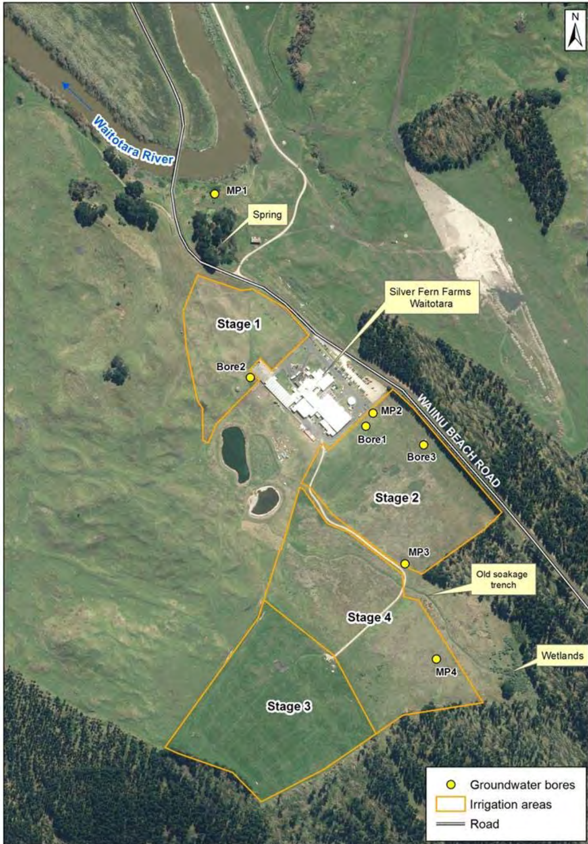
Figure 1 Location of SFF Waitotara meat processing plant showing irrigation areas and groundwater monitoring points
