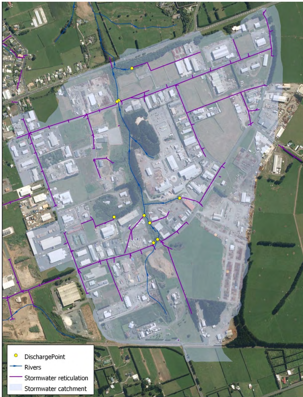
Figure 5 NPDC stormwater catchment, reticulation, and discharge points
