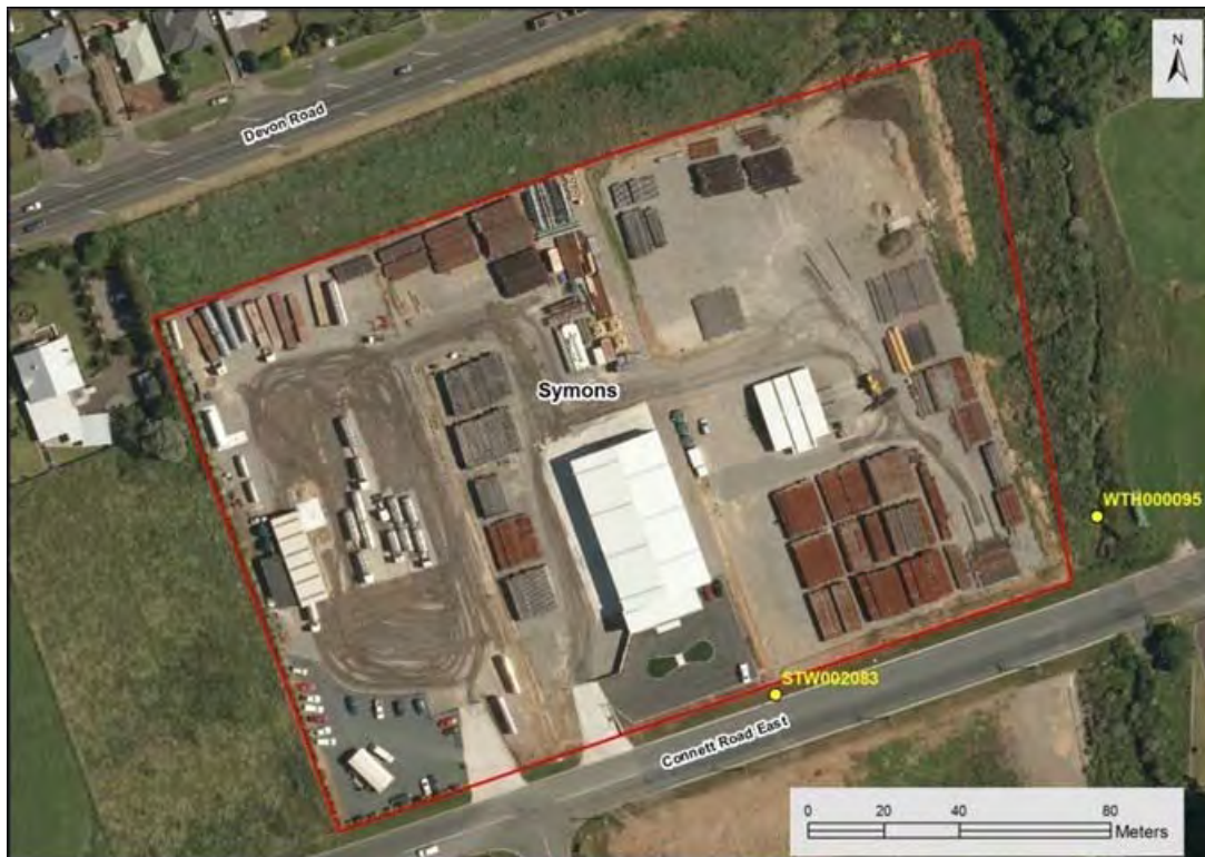
Figure 9 Symons' stormwater discharge sampling point and downstream site
