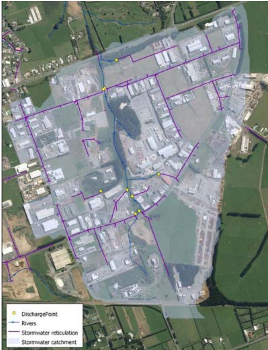
Figure 5 NPDC stormwater catchment, reticulation, and discharge points
