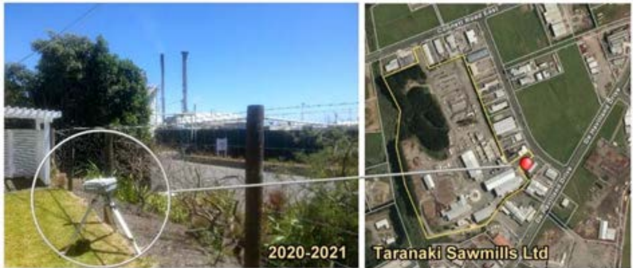
Figure 15 View of DustTrak PM10 monitor during deployment
