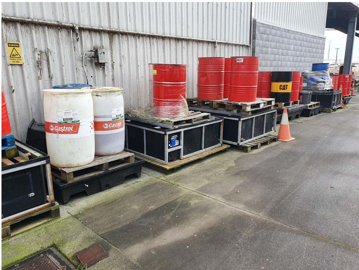
Photo 16 Bundling in place beside OMV wash facility, August 2018
