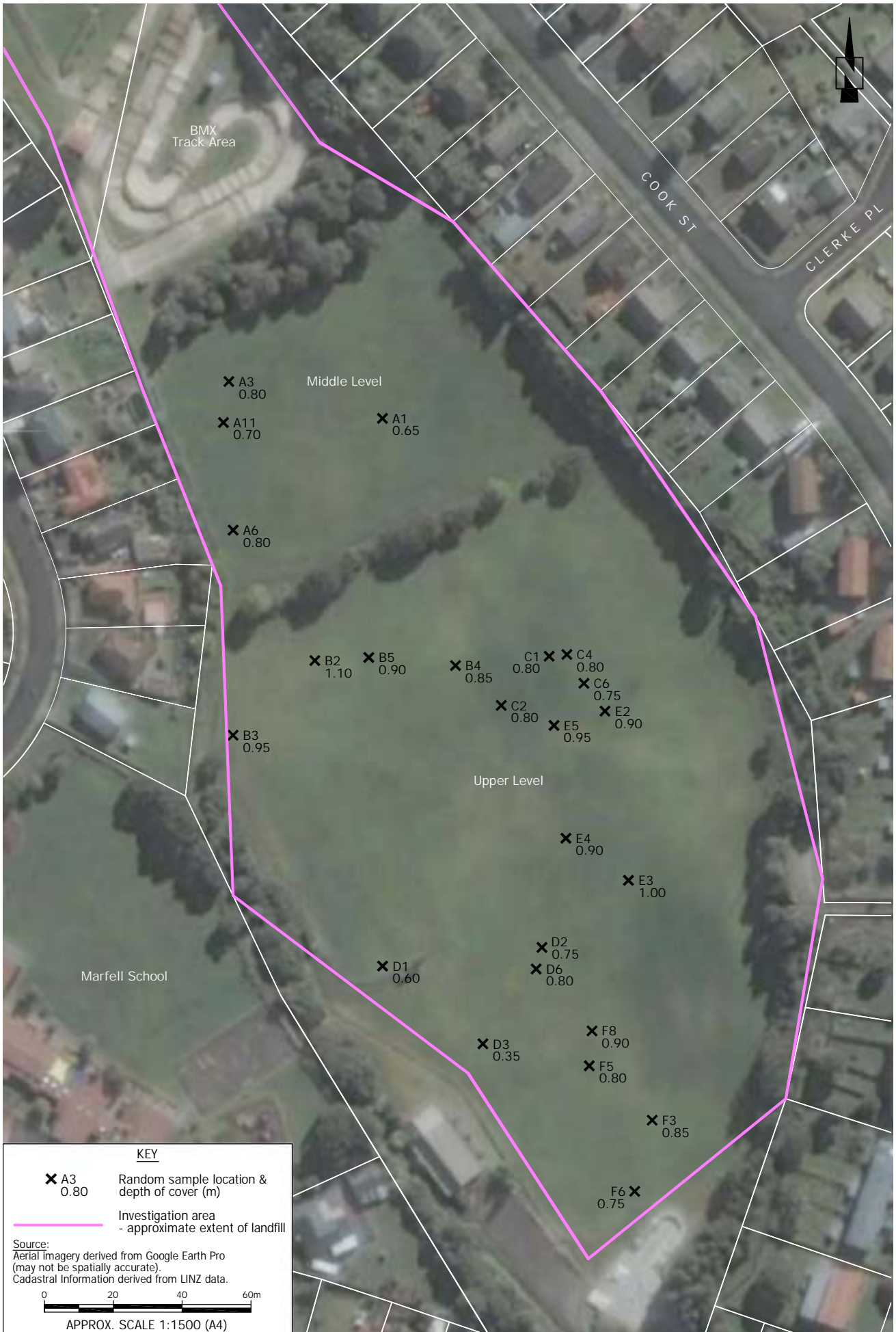
Figure 2 : DEPTH OF COVER (UPPER & MIDDLE LEVELS)
