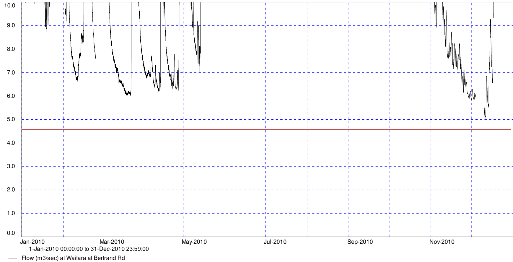
Magnified view of the hydrograph showing the flow of the Waitara River at Bertrand Road January to December 2010. The consent limit of 4.6m 3 /s is shown as a red line. At no point during 2010 did the flow in the Waitara River at Bertrand Road fall below 4.6m 3 /m.
