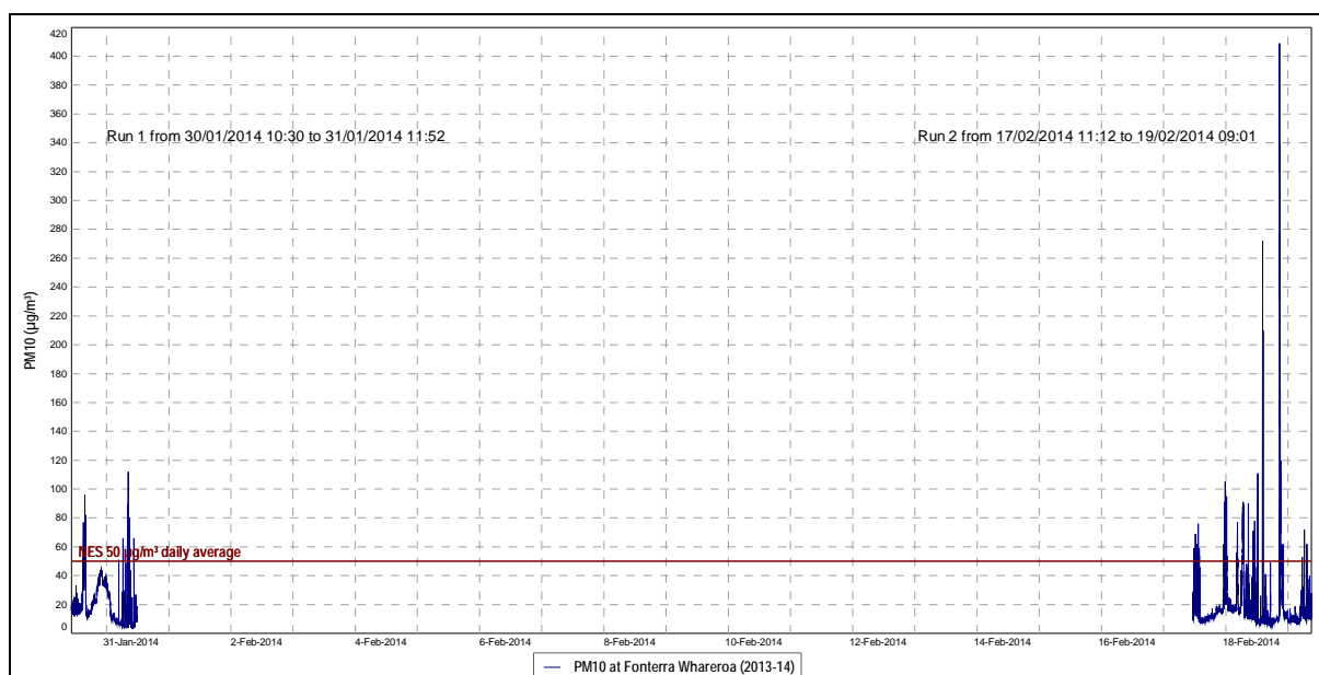
Figure 2 PM10 concentrations ( \mu\text{g}/\text{m}^3 ) at the Fonterra Whareroa dairy complex (2013-14)
