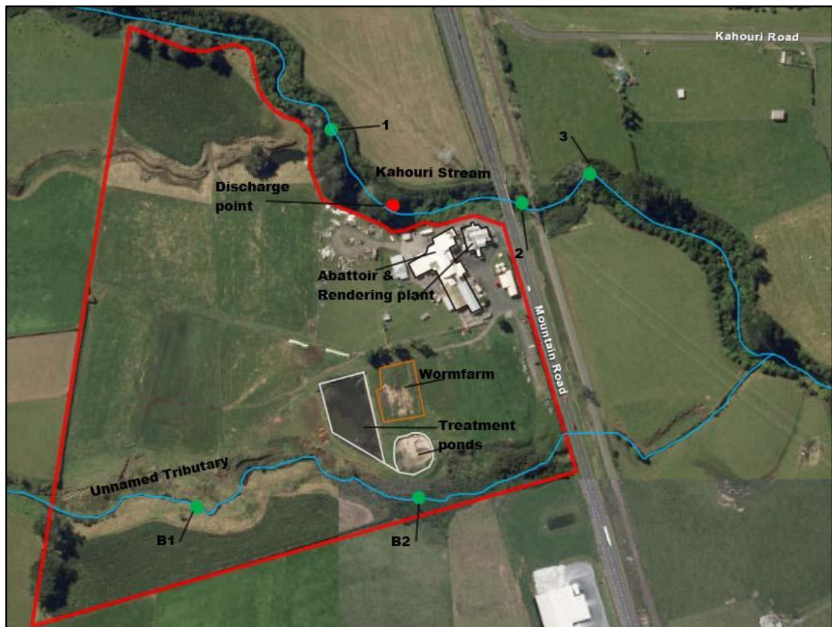
Figure 1 Taranaki Abattoirs site layout and biomonitoring sites, in relation to the discharge point
