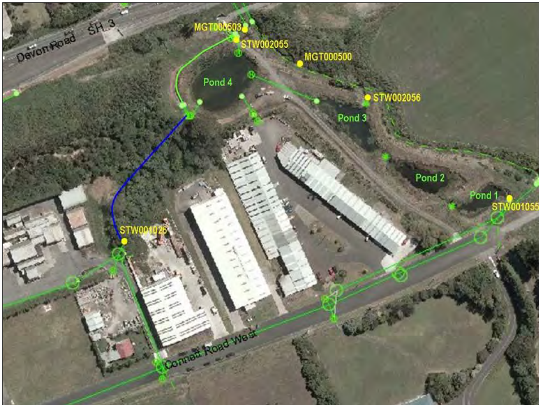
Figure 5 NPDC stormwater flow paths and sampling points
