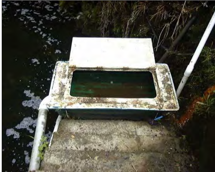
Photo 14 Elver trap at the base of the tail race at the power station
