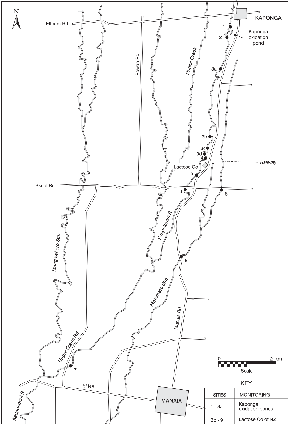
Figure 1 Biomonitoring sites in the Kaipokonui River sampled in relation to Fonterra Kapuni factory discharges
