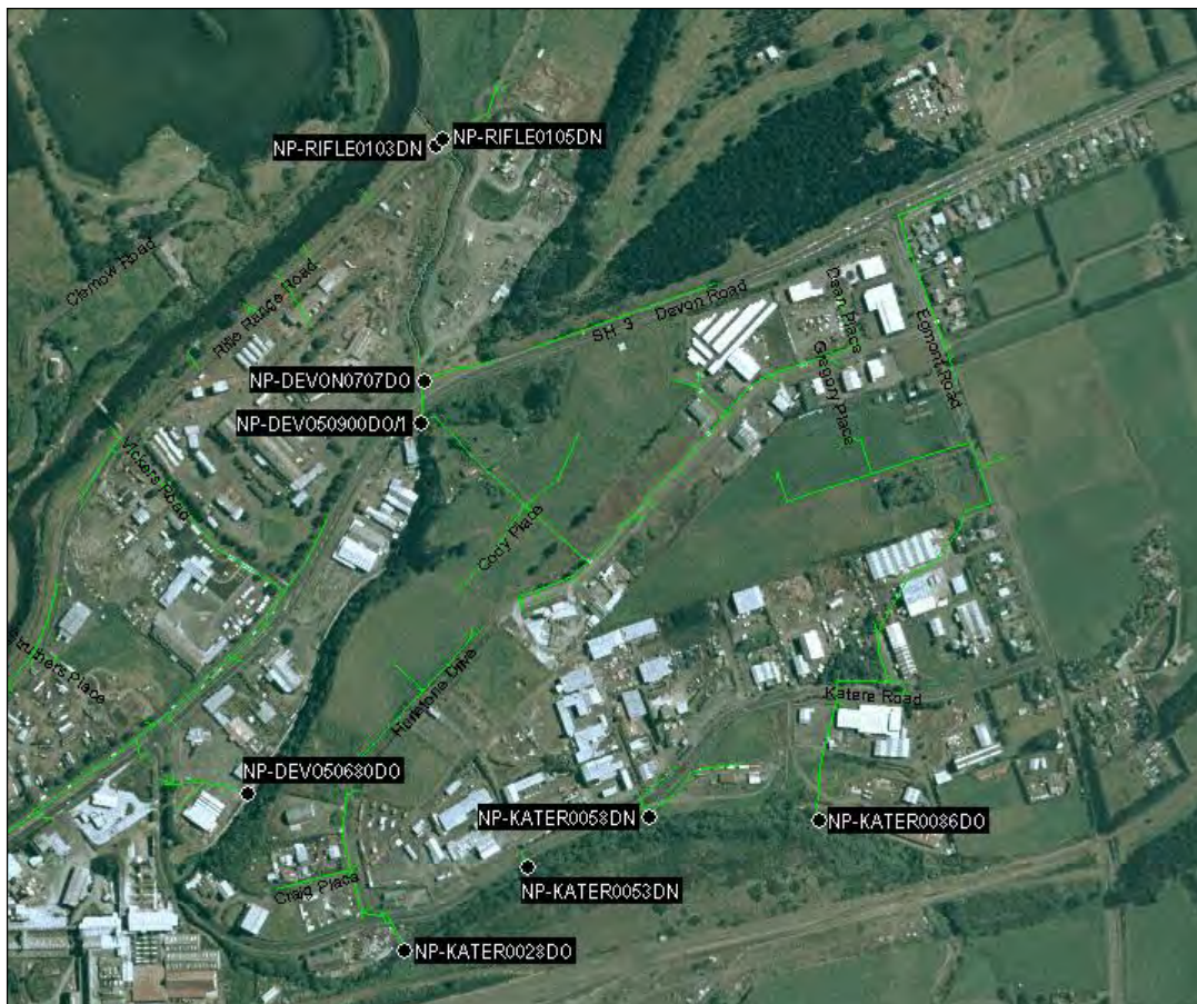
Figure 14 NPDC stormwater drainage and consented discharge points to the Mangaone Stream
