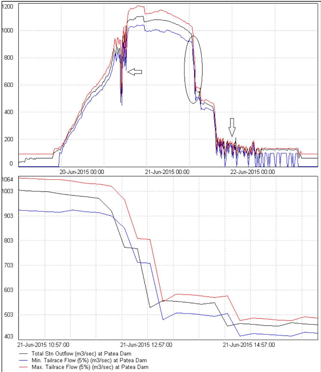
Figure 7 Total station outflow from 21 June to 23 June 2015, compared with maximum and minimum allowable flow. The arrows mark the times affected by short-term fluctuations in spill flow, while the circled area is expanded in the lower graph.
