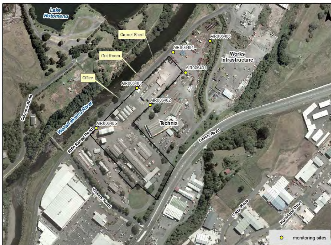
Figure 6 Fitzroy Engineering Group Ltd site and deposition gauge locations
