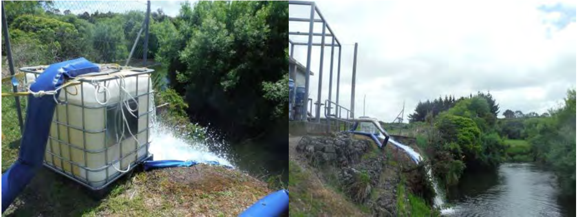
Photo 2 Intake fish entrainment trial, 27 November 2014
