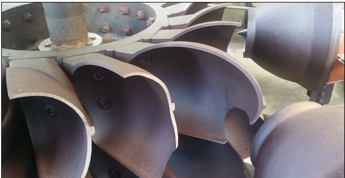
Photo 3 The damaged pelton wheel (below) and a jet containing large debris (right)
