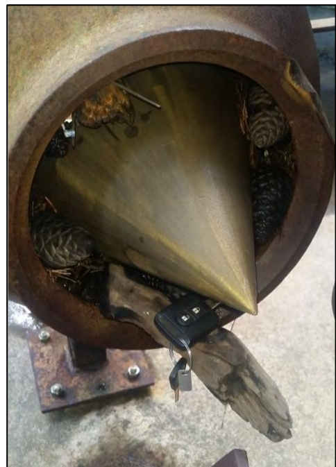
Photo 3 The damaged pelton wheel (below) and a jet containing large debris (right)
