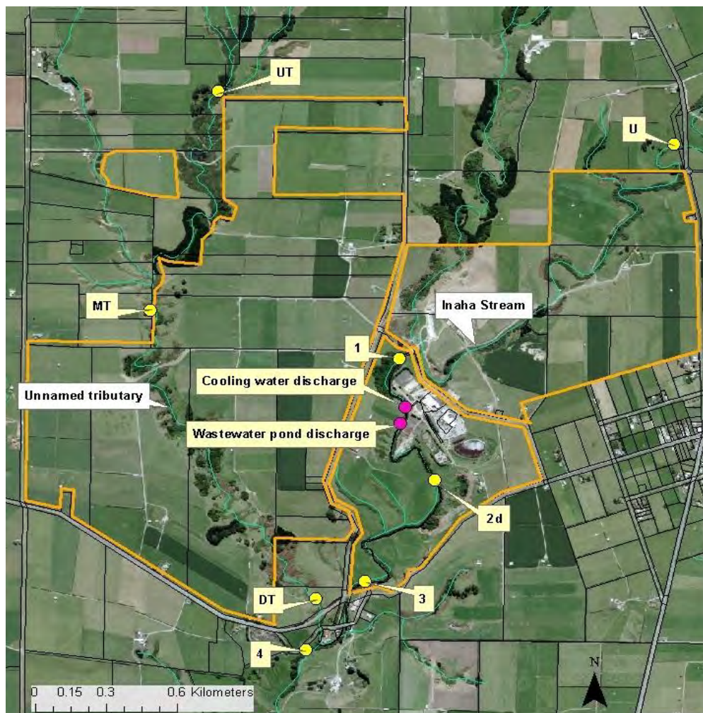
Figure 1 Aerial photo showing biomonitoring sites in the Inaha Stream and an unnamed tributary stream relating to discharges from the Taranaki By-Products plant. The orange line outlines the irrigation areas around the rendering plant.
