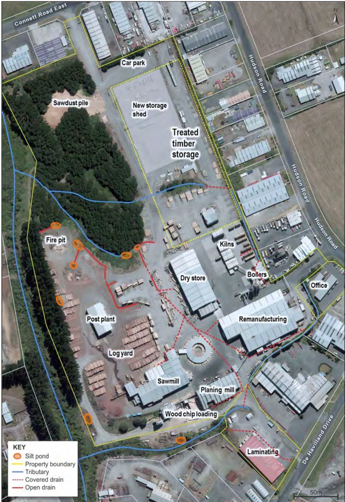
Figure 6 Taranaki Sawmills site drainage systems
