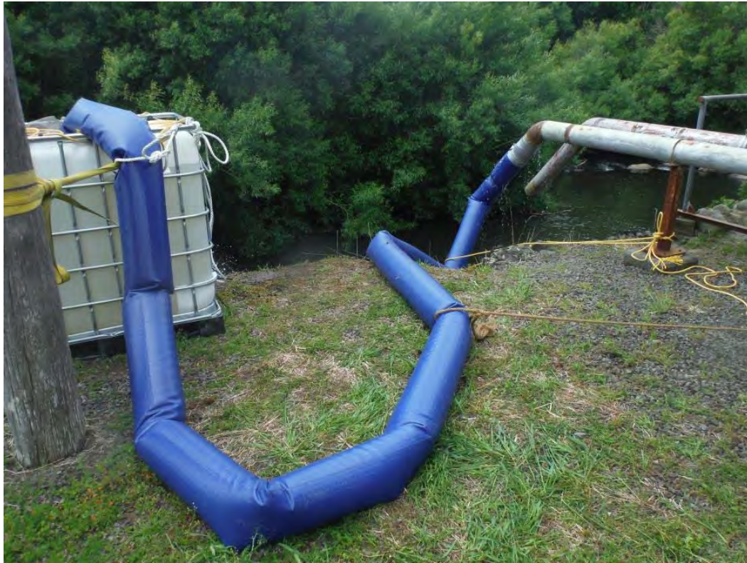
Figure 3. Hose leading from the outlet pipe to the container holding the net
