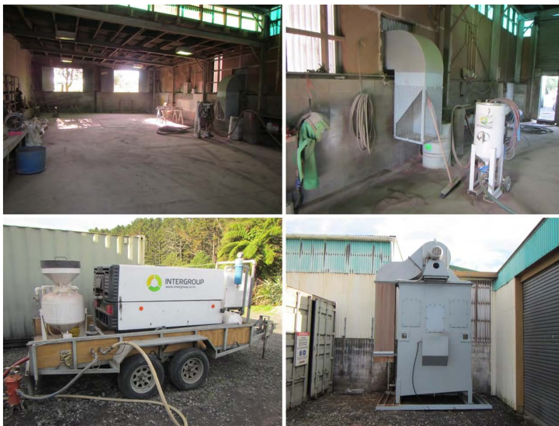
Photo 3 Site photos from Intergroup Ltd showing the blasting shed and key process equipment
