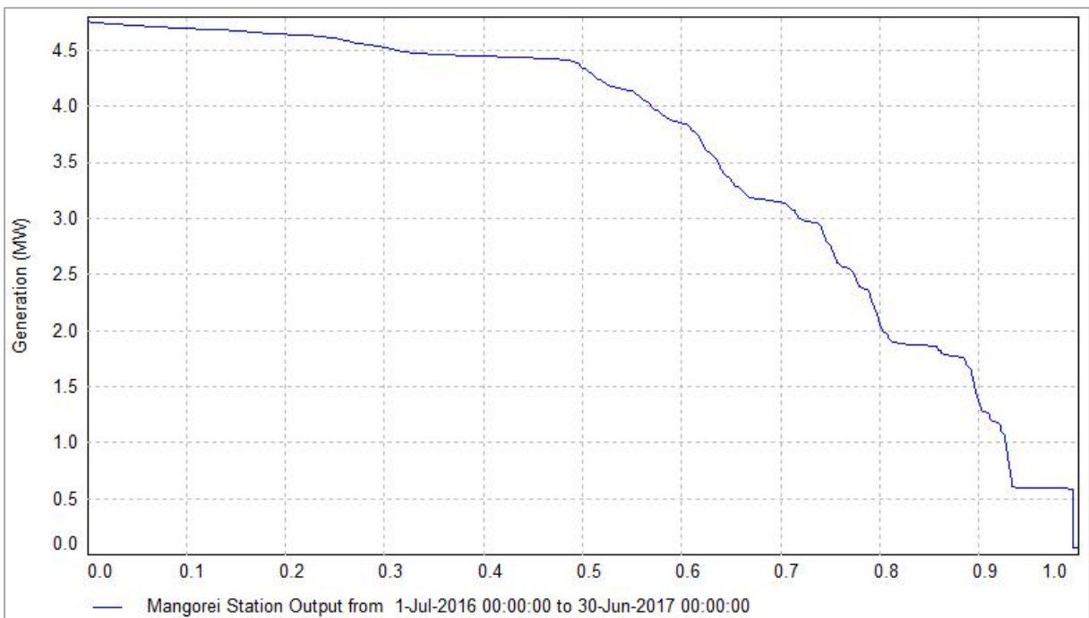
Figure 5 Generation at the Mangorei Power house, displayed as the percent of time a value was exceeded, 1 July 2016 – 1 July 2017, 9am to 5pm only
