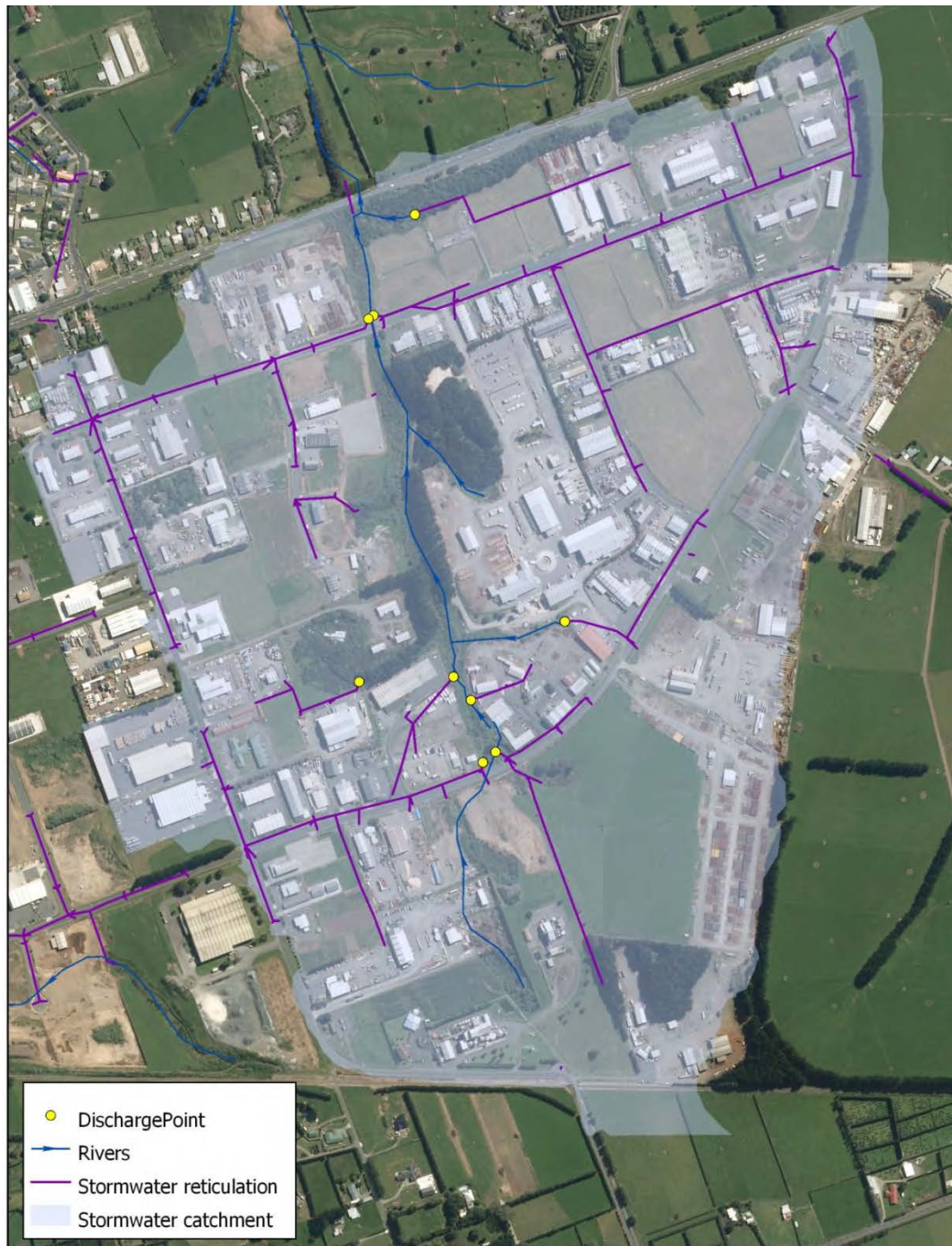
Figure4 NPDC stormwater catchment, reticulation, and discharge points
