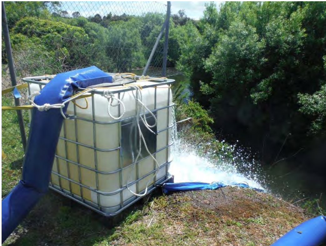
Figure 2. Sampling in operation at full velocity (75 m 3 /h)
