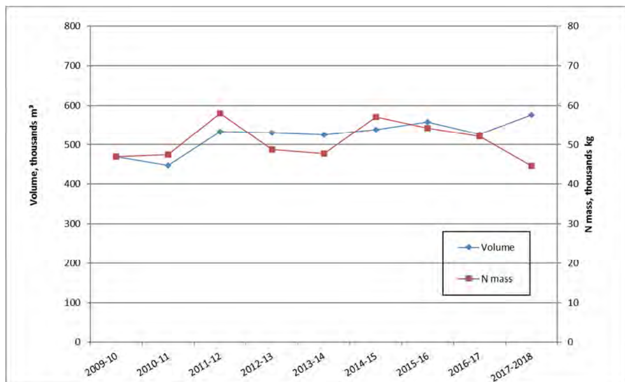
Figure 16 Annual volume of factory wastewater and estimated factory nitrogen mass irrigated, 2009 - 2017
