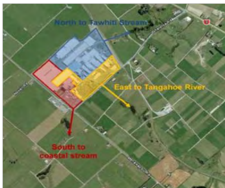
Figure 4 Approximate stormwater catchments at the Whareroa site
