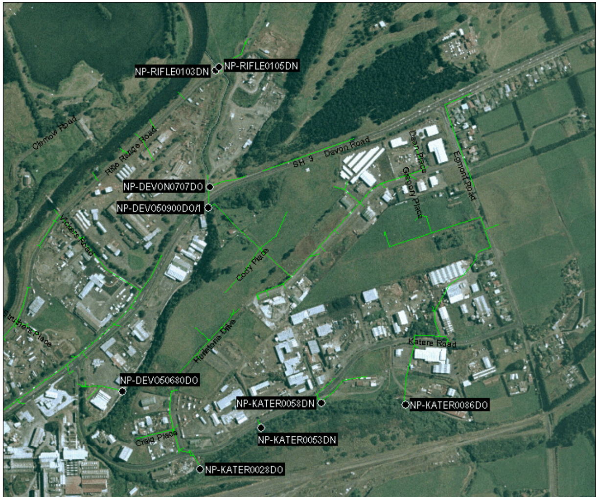
Figure 15 NPDC stormwater drainage and consented discharge points to the Mangaone Stream
