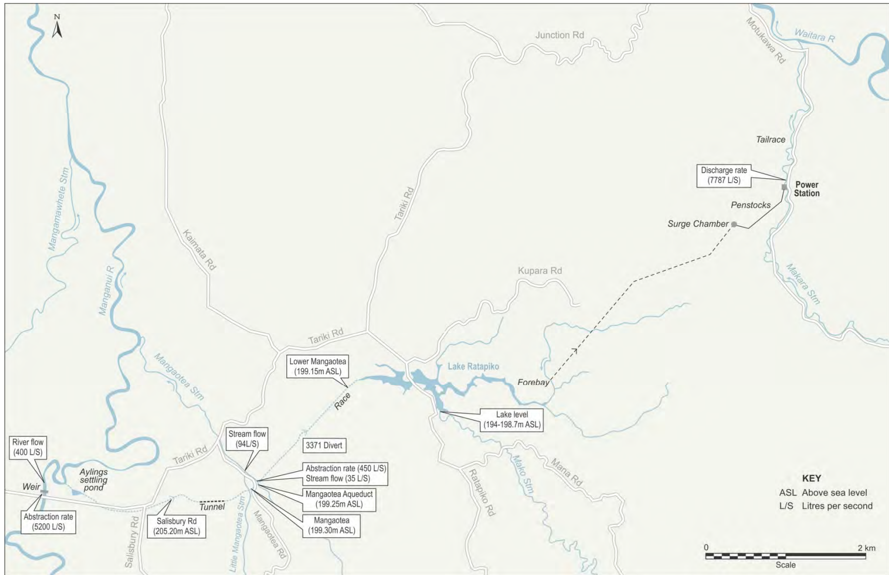
Figure 3 Location of water abstraction, discharge and water level monitoring sites for the Motukawa HEP scheme (limits in brackets)
