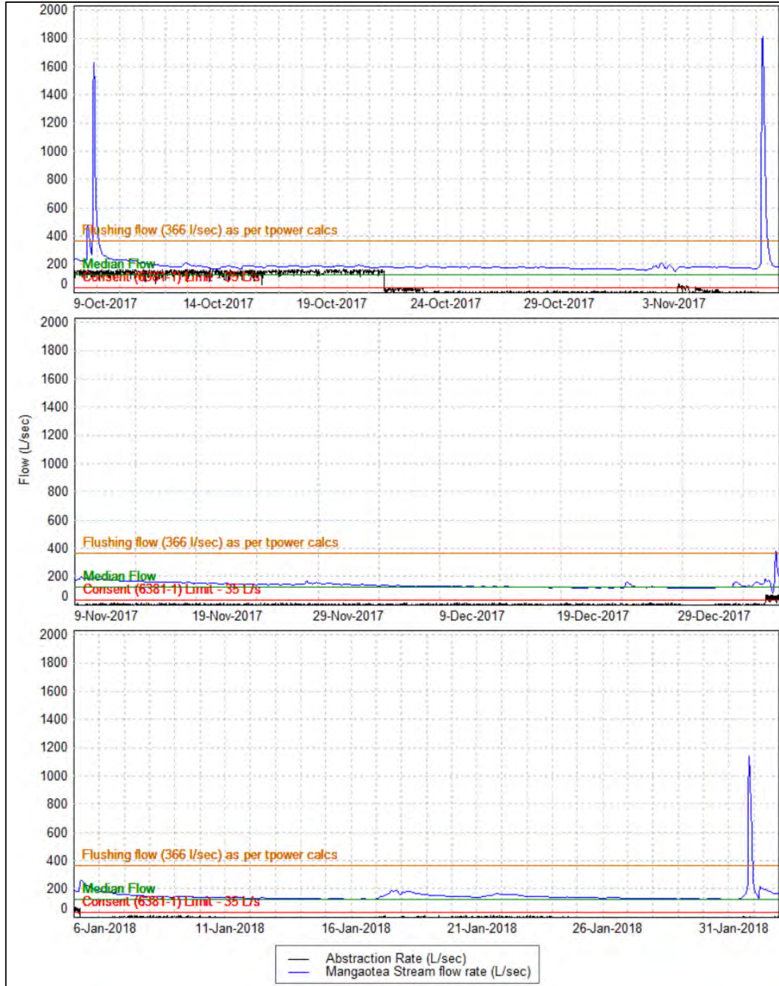
Figure 5 Flow rate in the Mangaotea Stream immediately downstream of the intake, and the abstraction rate from the Mangaotea Stream at a time when abstraction ceased as required (top), when abstraction started when flushing was required, and when abstraction seemed to continue (albeit at a low rate) during the natural flushing flow (bottom).
