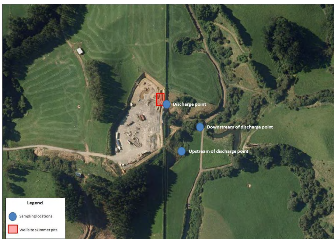
Figure 2 Stormwater and surface water sampling locations at the Cheal-B wellsite
