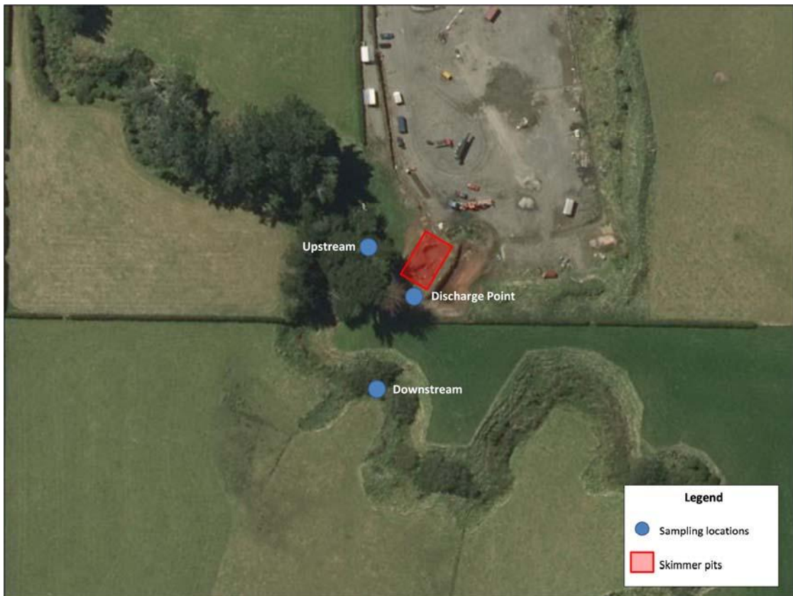
Figure 2 Stormwater and surface water sampling locations at the Cheal-C wellsite
