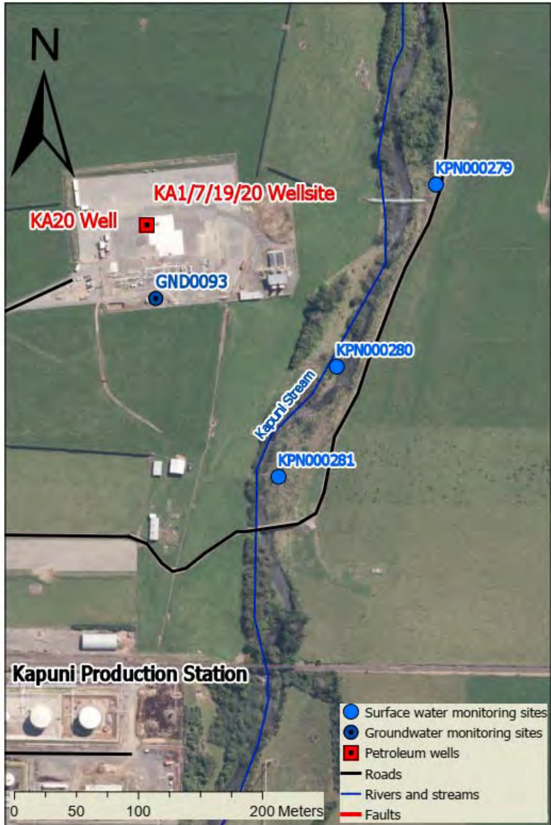
Figure 3 Surface water monitoring sites
