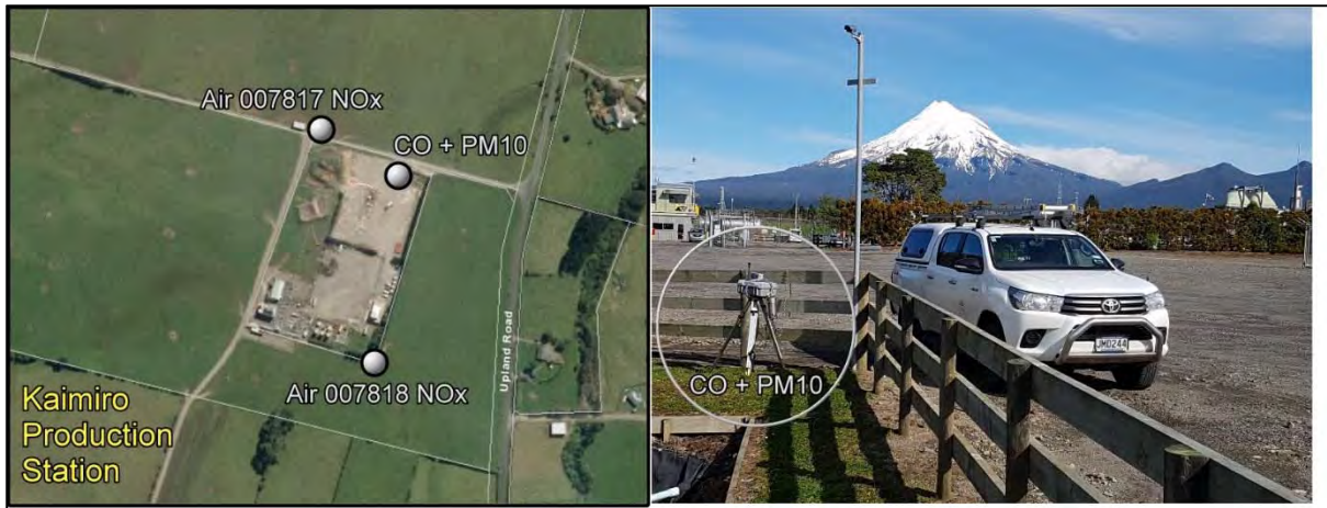
Figure 1 Air monitoring sites at Kaimiro production station (2017-2018)
