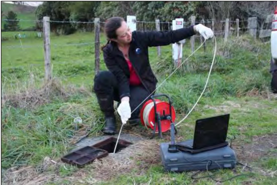
Photo 1 Measuring groundwater level at site GND0508
