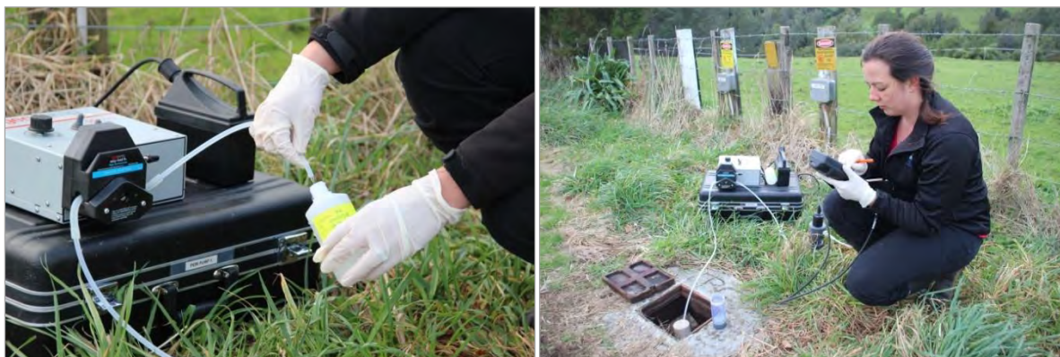
Photo 2 A staff member monitors field chemistry during purging of GND0508 and obtains a sample using a peristaltic pump
