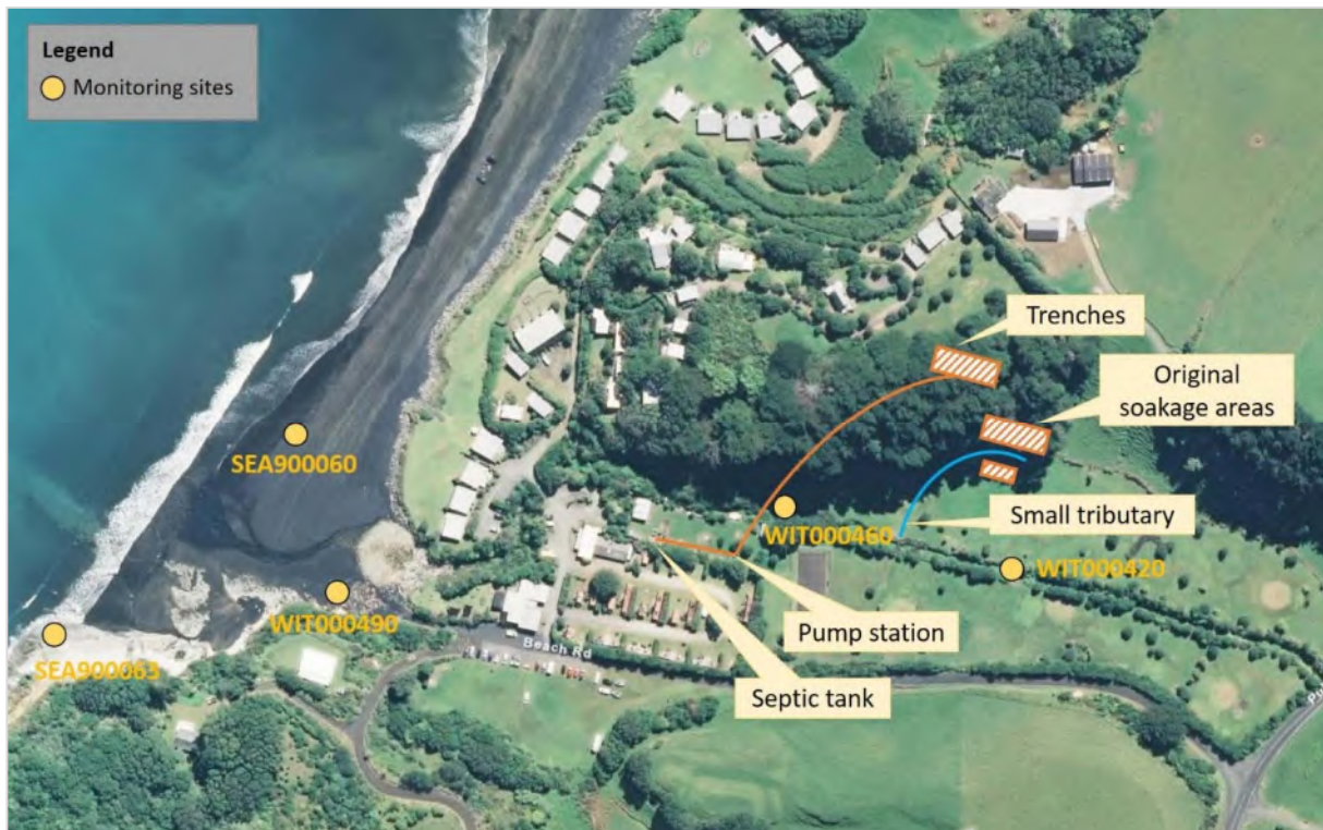
Figure 1 Locations of wastewater treatment system and sampling sites at the Wai-iti Beach Retreat
