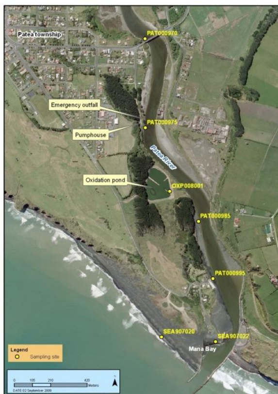
Figure 10 Aerial location map of sampling sites in relation to the Patea upgraded three cell oxidation pond system
