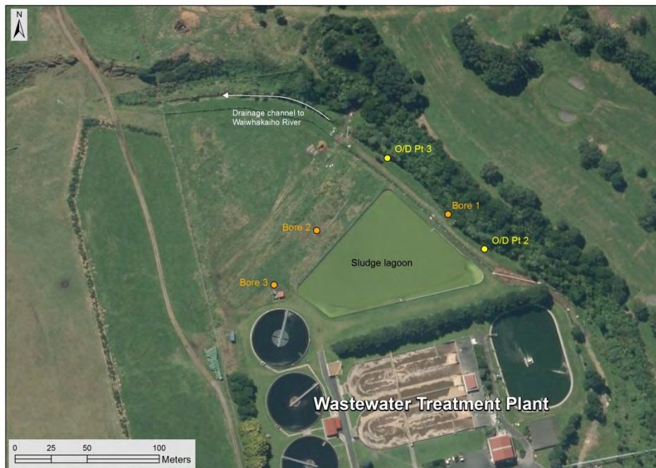
Figure 2 Sludge lagoon showing location of NPDC's groundwater bore and drain sampling sites
