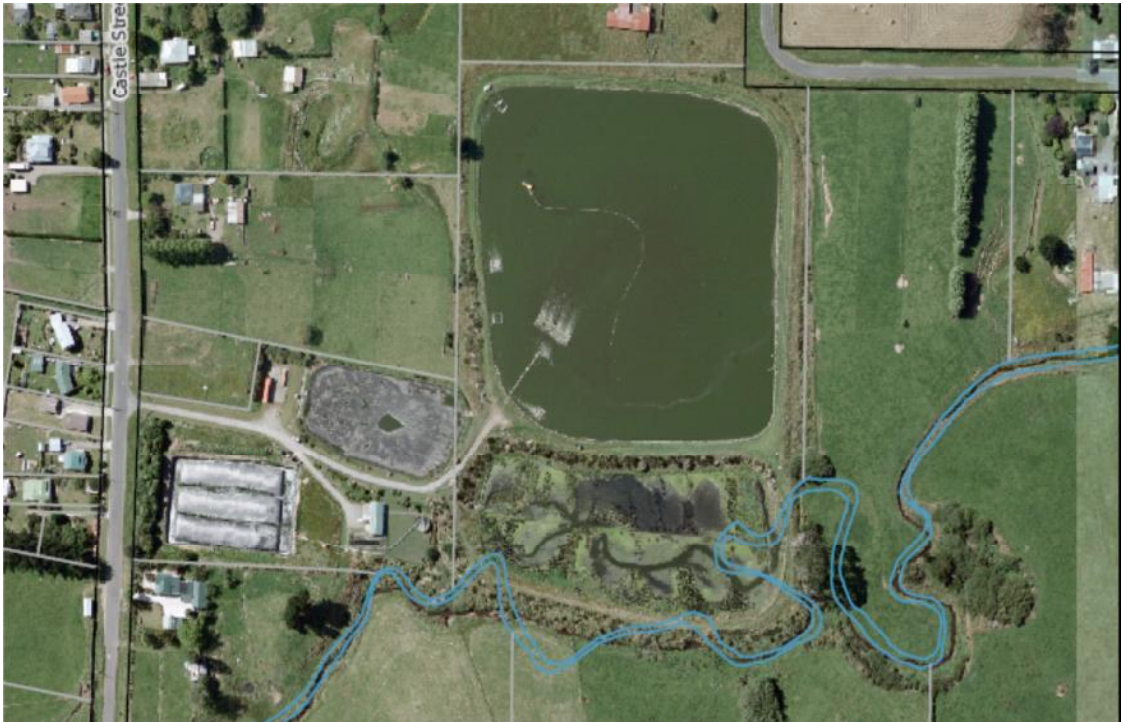
Figure 2 Aerial view of the Eltham WWTP showing the sludge geo-textile bags disposal area (lower LH corner) near the plant entrance [Note: the wetland (lower, centre) was converted to a holding pond in early 2011]
