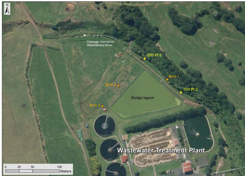
Figure 6 Sludge lagoon showing location of NPDC's groundwater bore and drain sampling sites
