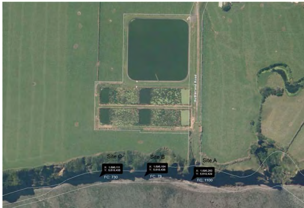
Figure 4 Sample sites in relation to wetland seepage at the Manaia oxidation ponds
